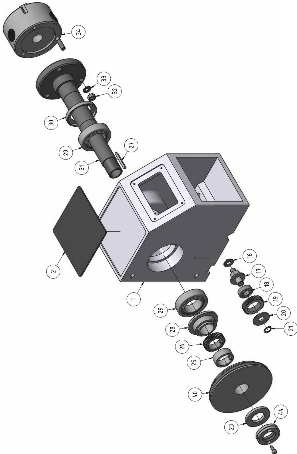
Abb.6-7: Spindelstock - Headstock
