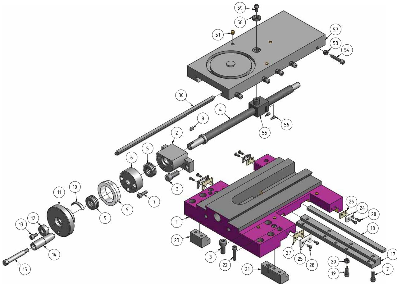
Abb.6-2: Planschlitten - Cross slide
